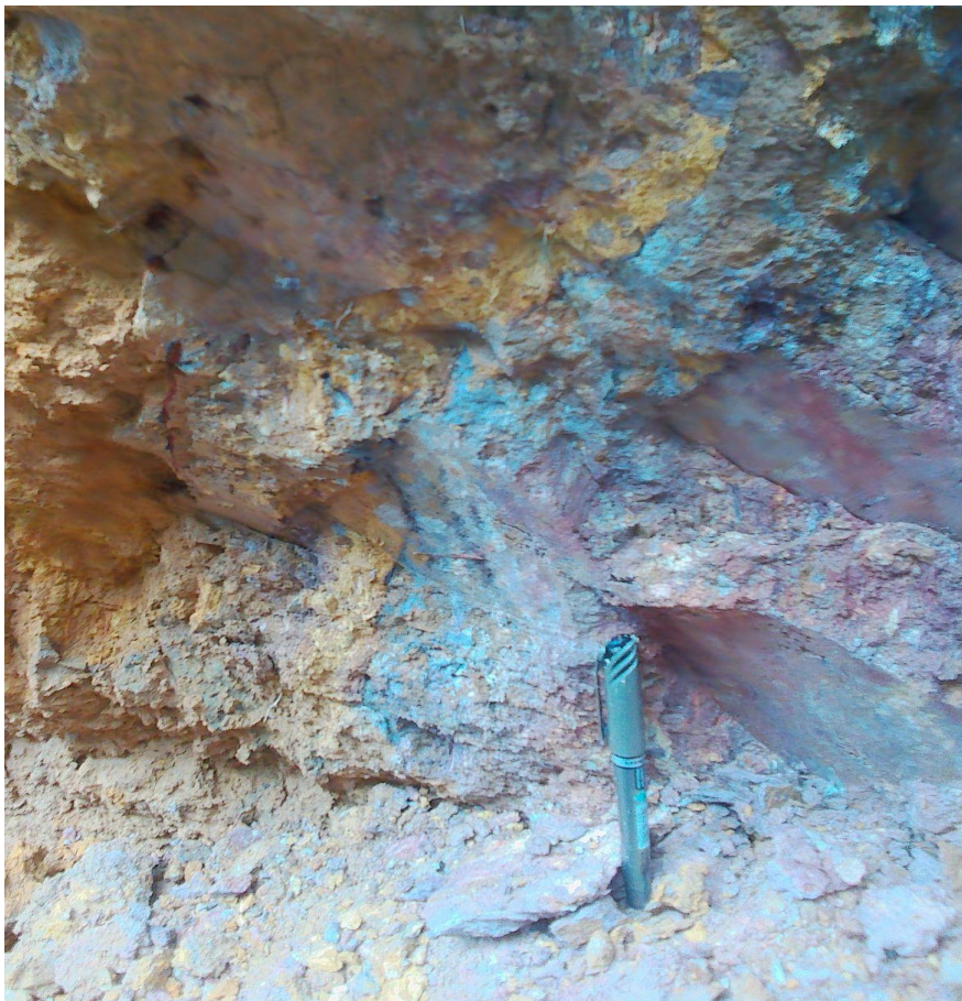
Figure 17. Example of saponite weathering in mafic volcanic rock with minor jarositic discoloration.
