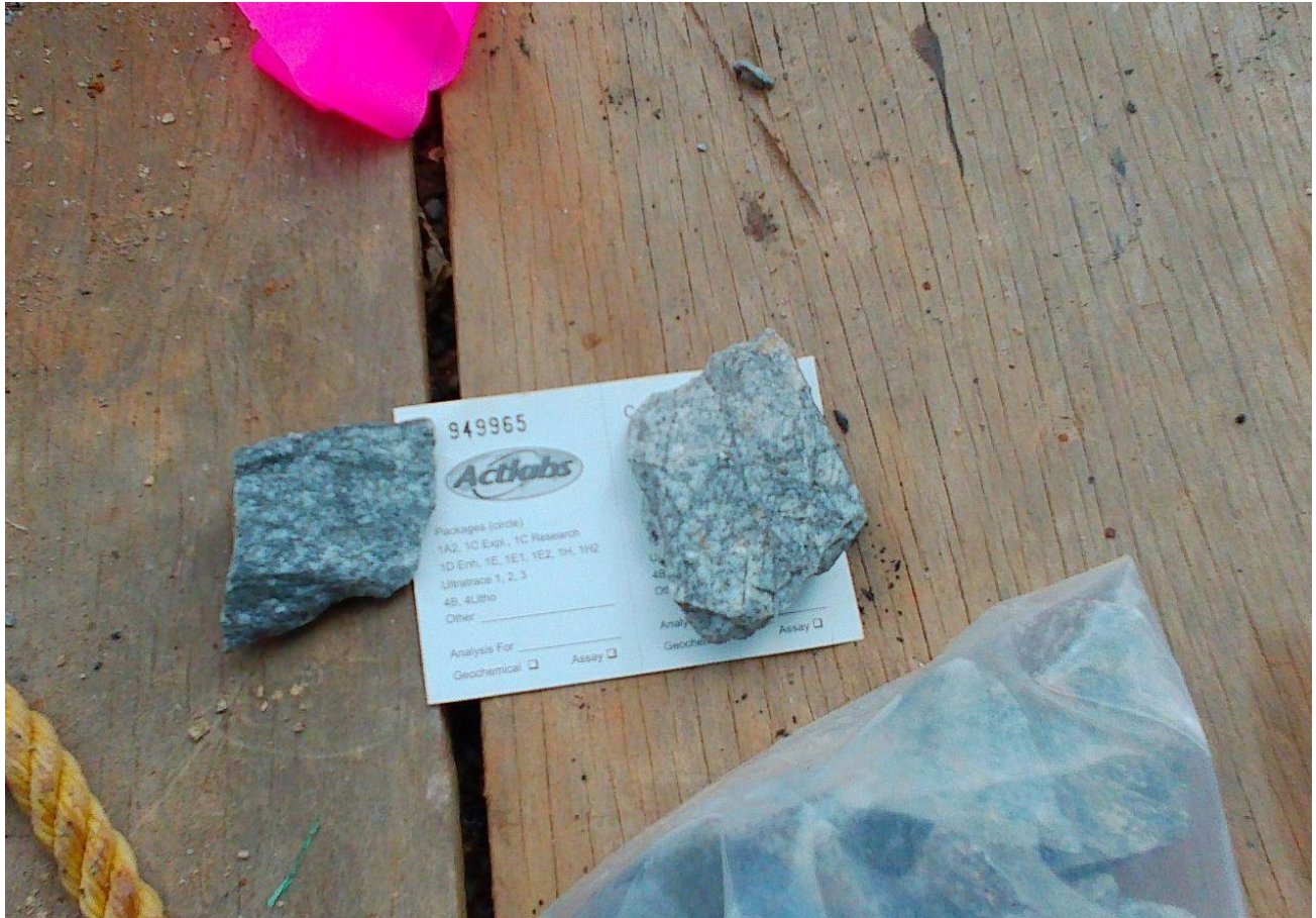
Figure 14. Sample C949965 showing representative brecciated wall rock with sericite slips and disseminated pyrite.
