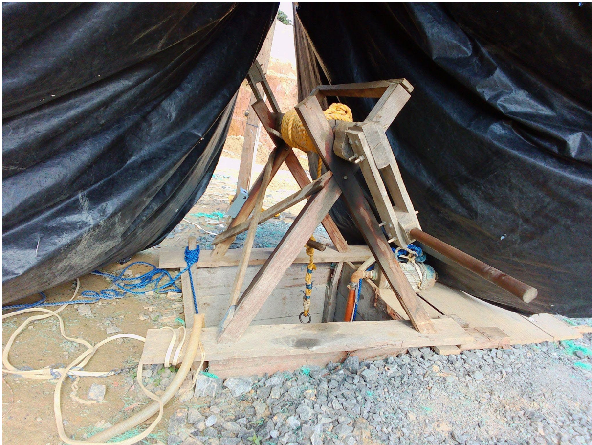
Figure 13. Manual hoist system constructed over inactive shaft.
