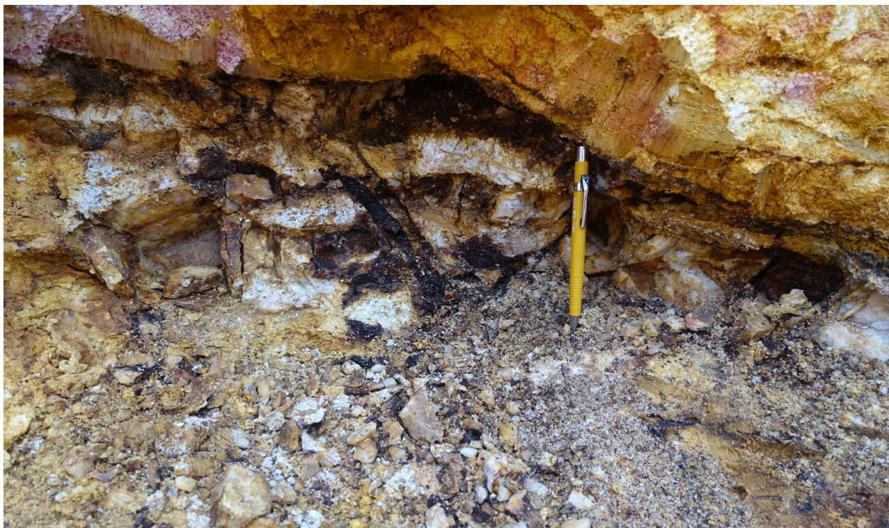
Figure 20. Sample C949974 showing sub horizontal quartz veining with minor FeOx staining along fractures and vein margins.
