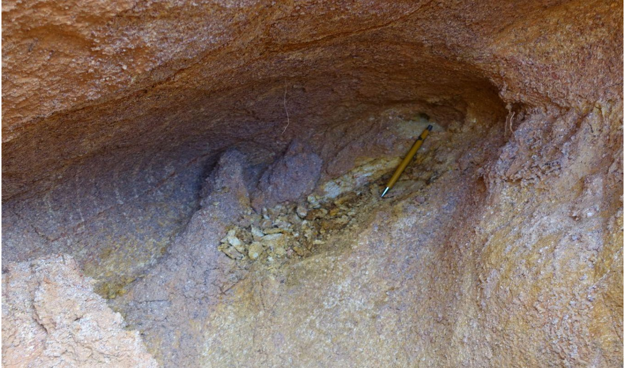
Figure 19. Sample C949972 showing sub horizontal quartz veining with minor FeOx staining along fractures and vein margins.
